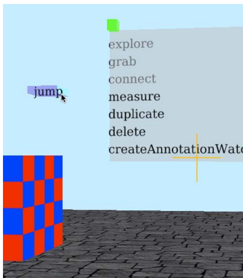
Figure 8. The "jump" menu item pulled off the menu for an object. The stand-alone jump item is not merely text, but still acts as a button which, when pressed, makes the original object jump.
