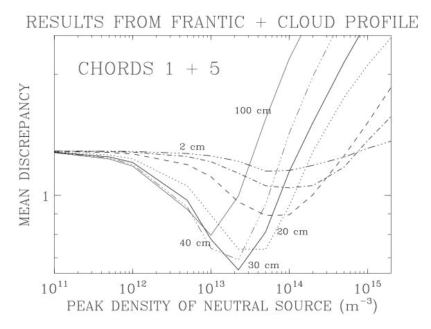
Figure 4-3: Optimization of the "FRANTIC+cloud" [H] profile, varying both the width and the peak density of the cloud, for n = 10. The 1/e cloud widths plotted are 2 cm, 6 cm, 10 cm, 20 cm, 30 cm, 40 cm, and 100 cm. The standard deviations of discrepancy are not shown on the plot.
