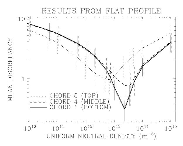
Figure 4-1: Optimization of the "flat" [H] profile for n = 10. The vertical bars represent  $\pm$  the standard deviation of the discrepancy. (See Section 4.1)
