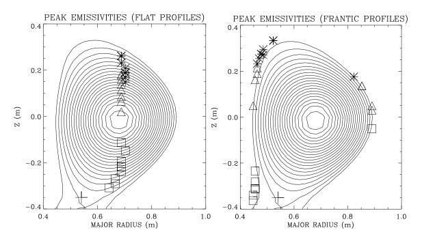
Figure 4-6: Locations of maximum charge exchange signal for the best fits to each chord position. Chords 1, 4, and 5, are plotted with squares, triangles, and asterisks, respectively.
