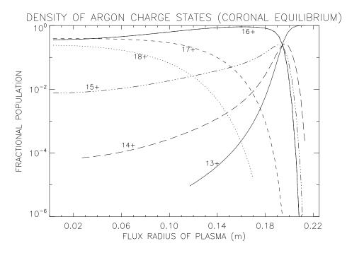
Figure 2-2: Calculated coronal equilibrium populations of Ar charge states as a function of equilibrium temperature, which ranges from 2600 eV at the center of the plasma to 0 at the edge.
