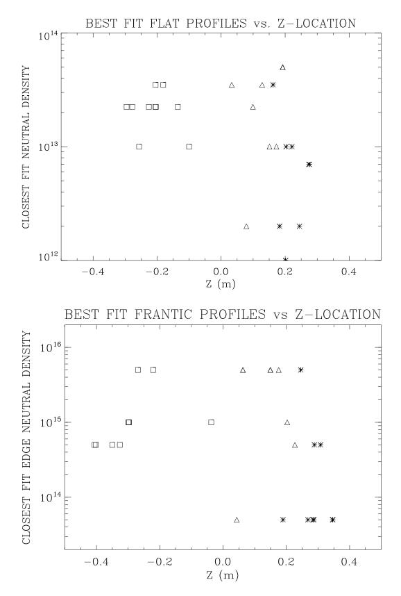
Figure 4-5: One - dimensional neutral profiles determined from matching a model to each of the scanned chord locations. Chords 1, 4, and 5, are plotted with squares, triangles, and asterisks, respectively.
