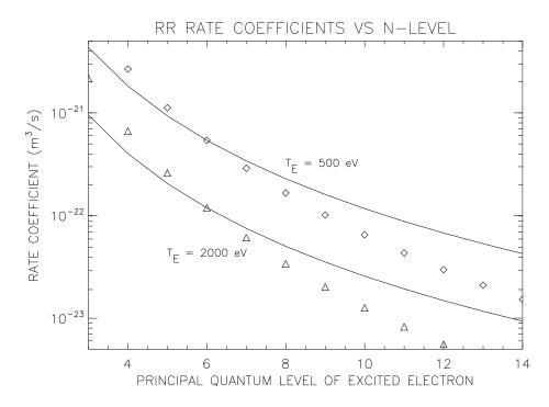
Figure 2-6: *n*-level dependence (diamonds and triangles) of the rate coefficient for radiative recombination of  $Ar^{17+}$  for two values of the electron temperature. The solid curves are  $1/n^3$ -shaped and pass through the value for n = 6. The discrepancy between the calculated rates and the  $1/n^3$  approximations is significant, especially when compared with a small charge exchange signal, and is temperature - dependent.
