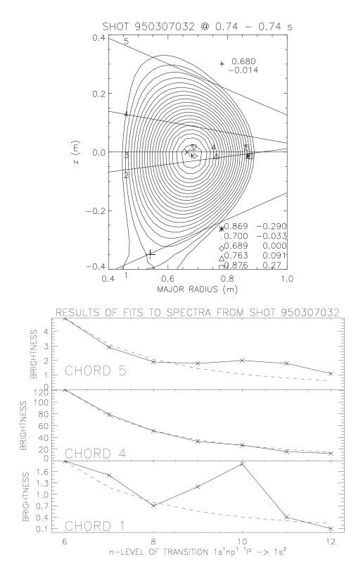
Figure 3-1: Cross-section through the plasma (TOP) showing the viewing angles of the HIREX chords for a particular plasma discharge. The signal observed is plotted vs. spectral line for three of the chords (BOTTOM). The dashed line is a  $\frac{1}{n^3}$  fit through the n = 6 datum.
