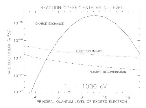
Figure 2-5: Rate coefficients for three processes which populate the  $1s^1np^1 - P$  state in  $Ar^{16+}$ , showing the different dependences on the level n.
