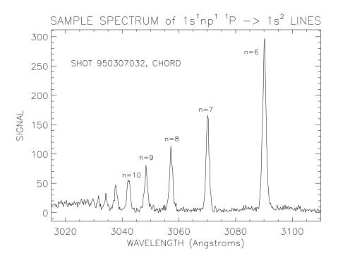
Figure 2-4: A portion of the  $1s^1n^1 - {}^1\mathsf{P} \to 1s^2$  spectrum with clearly resolvable lines in the range n = 6 to n = 14. Little or no enhancement of the  $n = \{9, 10\}$  lines is evident: the brightnesses fall off roughly as  $1/n^3$ .
