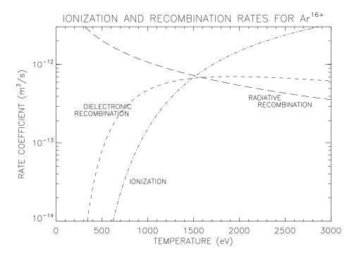
Figure 2-1: Ionization and recombination rate coefficients versus temperature, shown for  $\mathsf{Ar}^{16+}$  .
