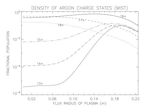
Figure 2-3: Calculated Ar charge states based on ionization, recombination, and transport processes.
