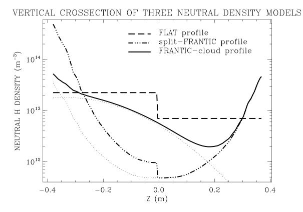
Figure 4-4: Cross-section through the [H] profiles for each of the three models used. The cross-section is along major radius 0.68 m (see Figure 3-1). The dotted lines show the two components of the FRANTIC+cloud distribution.
