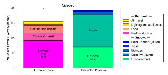
The stack on the left shows the sum of all energy currently consumed, as both electricity and combustion, in Quebec. On the right is a breakdown of available renewable energy resources.
