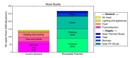
The stack on the left shows the sum of all energy currently consumed, as both electricity and combustion, in Nova Scotia. On the right is a breakdown of available renewable energy resources.
