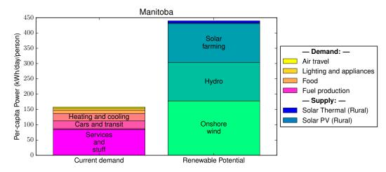
The stack on the left shows the sum of all energy currently consumed, as both electricity and combustion, in Manitoba. On the right is a breakdown of available renewable energy resources.
