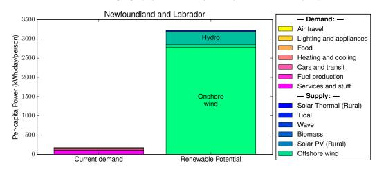
The stack on the left shows the sum of all energy currently consumed, as both electricity and combustion, in Newfoundland & Labrador. On the right is a breakdown of available renewable energy resources.
