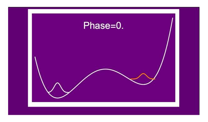
This animation shows the double well with part of an electron in each side. This graphic shows how the qubit stores two real numbers at the same time.
