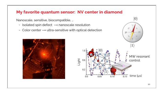
What are practical sensors? You might already be familiar with atomic clocks. Other modalities include for example spin defects in diamond. These emit red light, that we can see by masking the green laser excitation. Like the needle of a compass, the spins orient themselves with external magnetic field, and their rotation from up to down (and superpositions, that we detect optically) indicate the strength of external magnetic fields.
