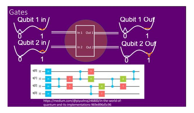
The top shows a gate - a set of interactions that take place for a time between two qubits. The calculation takes place in the qubit, in contrast to a classical computer where data moves in and out of memory to a central processing unit where calculations take place.
