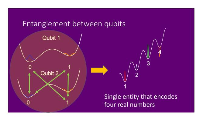
The two qubits form a single system with four wells, encoding four real numbers encoded in the phases and amplitudes. You might think the sytem can encode eight numbers, but keep in mind the amplitudes describe two electrons spread over the four wells, so there are four amplitude and phase relations. From this we can sumerize that adding a qubit to the system doubles the number of real numbers the system can hold. Adding one qubit to these two would would store eight numbers, and so on.
