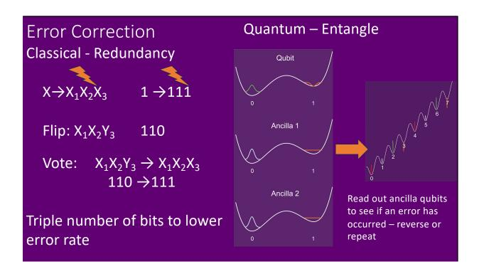
From the beginning, designers had to contend with "bit flips" from electrical noise or cosmic rays. Much of the most sophisticated electronics in our computers today contend with error correction. Majority voting provides the simplest method, shown here. Our computers use much more eifficient error correction schemes.
