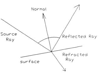
parameters. A specularly reflected (or refracted) ray is distributed in a cone with an angle theta and according to a cosine to the power n law. These four numbers are theta, n for reflection and theta, n for refraction respectively. If you want to add your own attributes, we recommend making these numbers "60 4.0 60 4.0."
