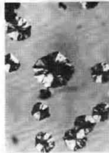
Figure 10 Micrograph from the mattock-head shown in figure 9. Unetched, crossed nicols. This micrograph was kindly supplied by Dr. Guan Hongye of the Foshan SG-iron Research Institute in Foshan, Guangdong.
