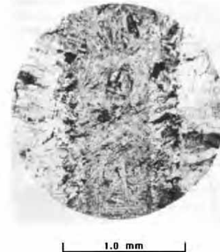
Figure 7 Micrograph from the hoe-head fragment shown in figure 6. (Li Zhong 1975, plate 1.5). Etched with nital.
